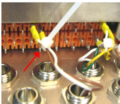
8. Secure the wires with a cable tie.
