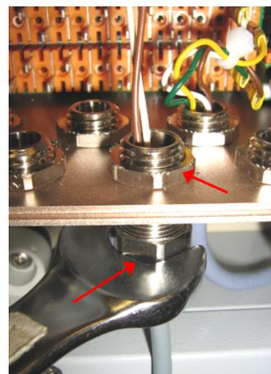
6. Tighten the nut with a wrench to secure in place. It may be necessary to use a second wrench to hold the top nut in place.
