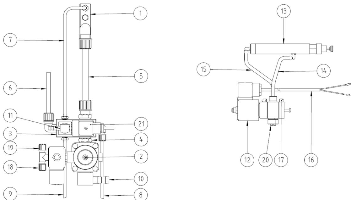
In the above illustration the rinsing system is shown on the left and the dilution system on the right.
