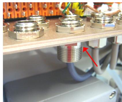
3. Screw the threaded part into the electronic unit opening selected in step 1 using the nut removed in step 1 to secure in place.
